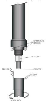
4. Whit the sensor facing down screw the cap clockwise to the end of the threads. Some electrolyte will overflow.
